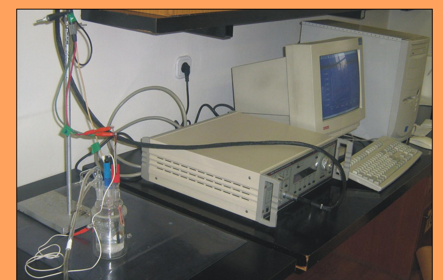
Fig. 7. Device setup for potentiodynamic measurements
